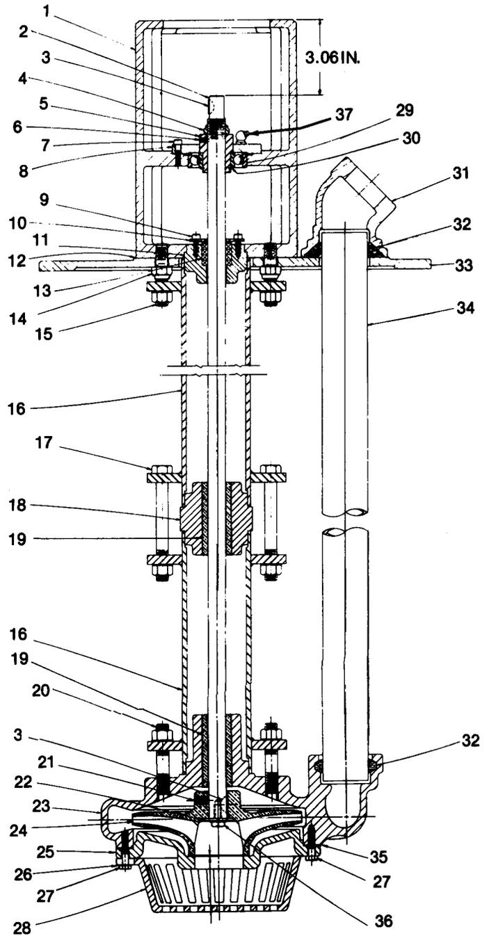
ADJUST NUT ITEM NO. 4 TO OBTAIN 0.012" TO 0.015" CLEARANCE BETWEEN IMPELLER AND SUCTION CASING
