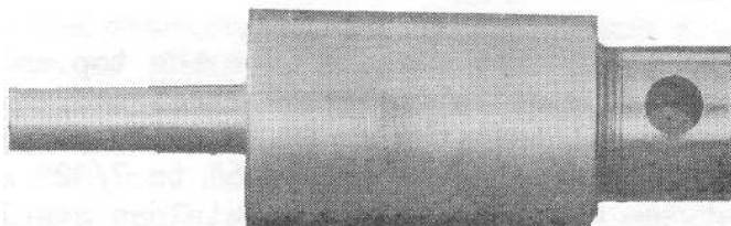
Figure 4 BEATER. For driving split-tapered impeller lock into impeller.
